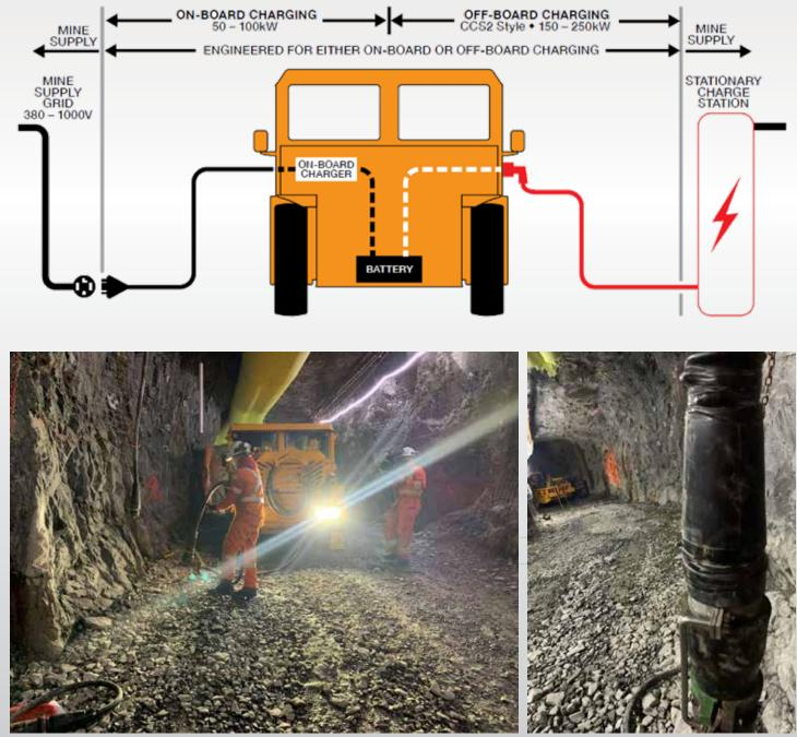
The charge rate depends on the capacity of the charger and the battery's capability to accept the charge. MacLean equipment can receive charges between 100-250kW.
