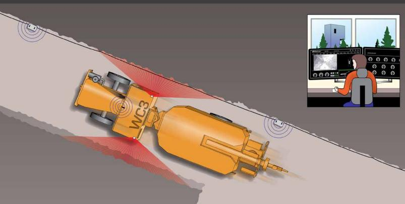
Control of all machine functions performed from an office-based operator station at the mine site or remote location.
